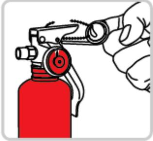
Place the extinguisher on the floor. Hold it by the tank (pressure on the handle could pinch the pin). Pull the pin
